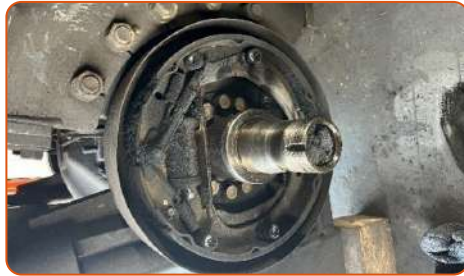
Current Condition: #618 Forklift: Abnormal brake operation and excessive wear of brake shoes.
