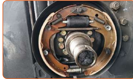
Corrective Action: Brake shoes replaced.
